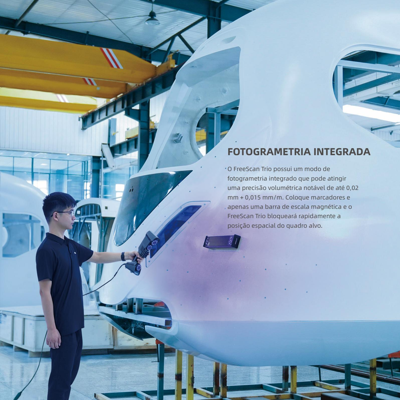
A man in a black shirt and glasses is using a handheld 3D scanner on a white car body in a factory. The scanner is emitting a blue light. The car body is mounted on a yellow and black stand. The background shows a large industrial building with yellow beams and a glass wall.
